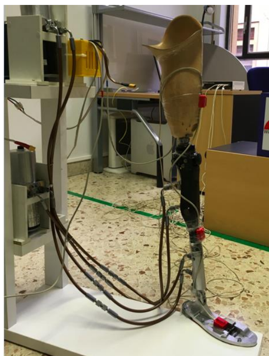
Fig.4. Above-knee prosthesis with separate hydraulic units and double-acting cylinders [9]
