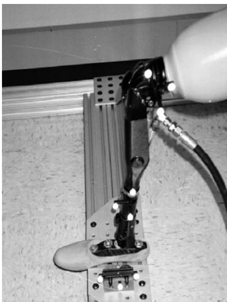
Fig.1. The first prototype of a hydraulic actuator-based above-knee prosthesis [4]
