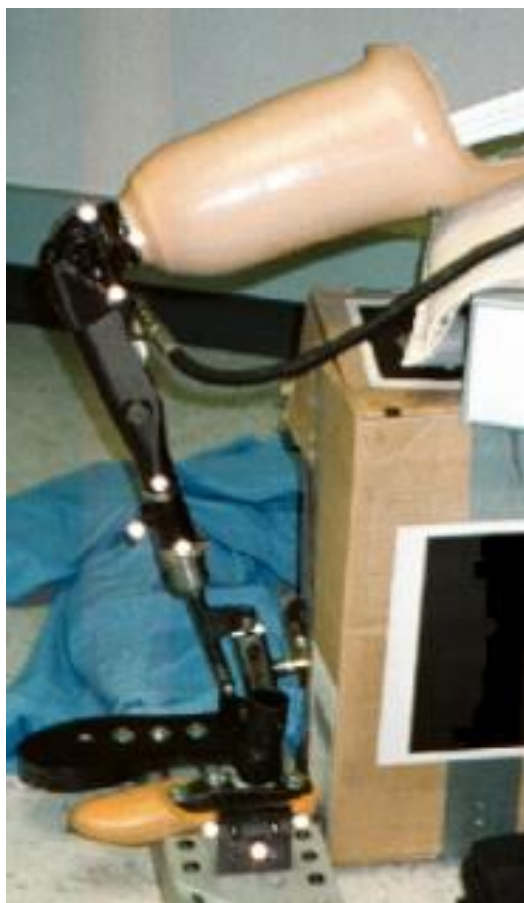
Fig.2. Improved above-knee prosthesis with an additional hydraulic cylinder in the ankle joint [7]
