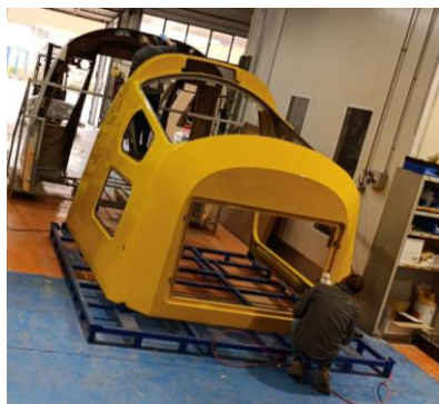
Fig.1. Tram's cabin preparing for transport after production
