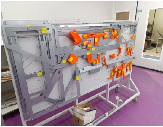
Fig.9. Sheet metal and additively manufactured fixtures
